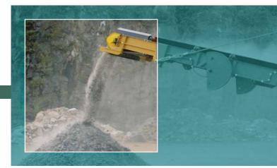
The Screening Plant is the most economic solution for screening of high-quality defined grain sizes. The screening plant can be operated by one person and is also available with a wireless remote control. All maintenance jobs can be quickly and easily performed, thanks to perfect accessibility.
